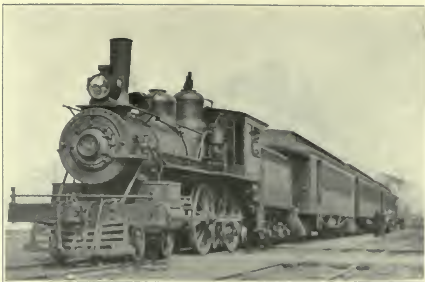
FIG. 371. SUBURBAN PASSENGER TRAINS. Suburban Train of the Chicago, Rock Island & Pacific Railway at Brainerd Station. This train consists of an American type locomotive and three coaches.
